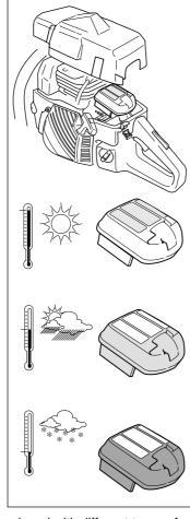
A Jonsered chain saw can be equipped with different types of airfilter according to working and weather conditions, season etc.
